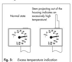
The temperature will exceed the adjusted limit if the valve cannot close due to dirt particles lodged between the seat and plug or due to a defective bellows. In this case, the excess temperature safeguard responds (see Fig. 5). The stem projecting out of the housing indicates a malfunction.
