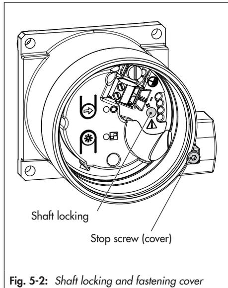
Fig. 5-2: Shaft locking and fastening cover
