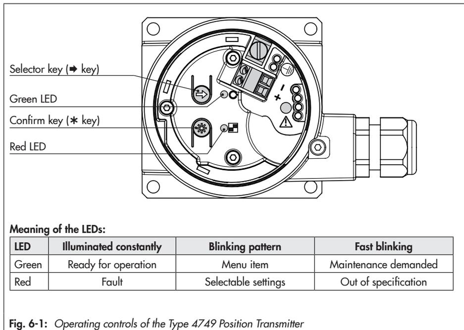
Fig. 6-1: Operating controls of the Type 4749 Position Transmitter
