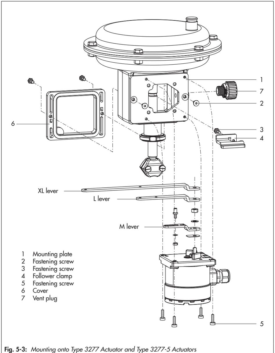
Fig. 5-3: Mounting onto Type 3277 Actuator and Type 3277-5 Actuators
