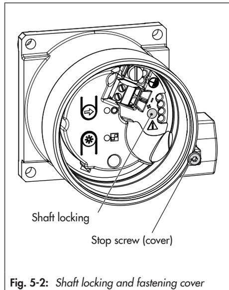
Fig. 5-2: Shaft locking and fastening cover
