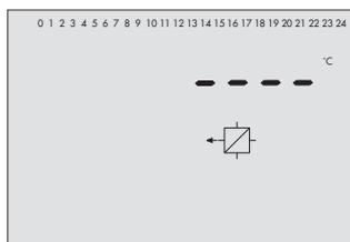
Return flow temperature at sensor RÜF or RÜFprim
