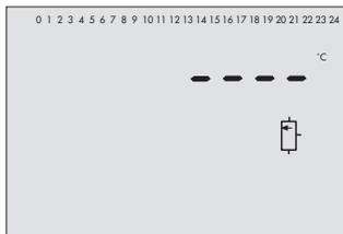
Storage tank temperature at sensor SF1
