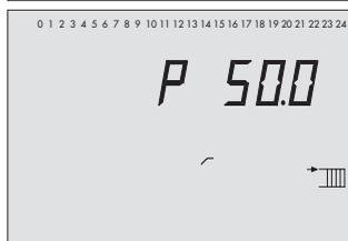
Maximum capacity of the heating
