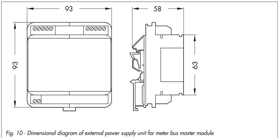
Fig. 10 · Dimensional diagram of external power supply unit for meter bus master module
