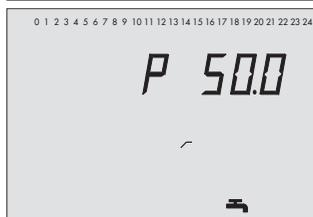
Maximum capacity of the DHW heating
