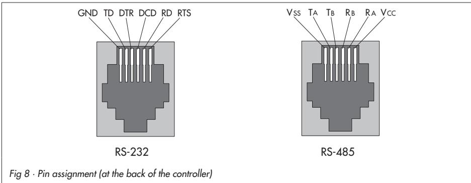
Fig 8 · Pin assignment (at the back of the controller)
