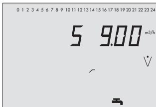
Maximum flow rate of the DHW heating
