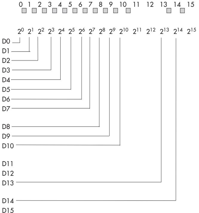
The holding register 258 can only be read over Modbus.
