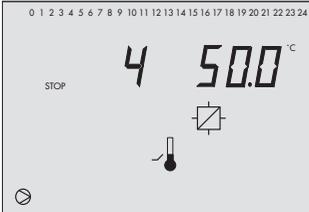
Heat exchanger charging pump, deactivation limit
