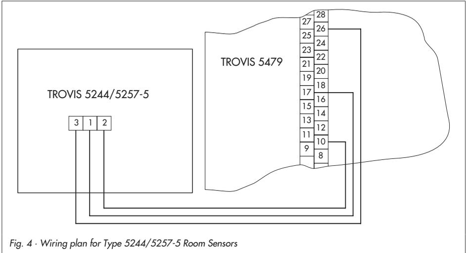
Fig. 4 · Wiring plan for Type 5244/5257-5 Room Sensors
