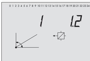
Gradient of the heating characteristic, return flow
