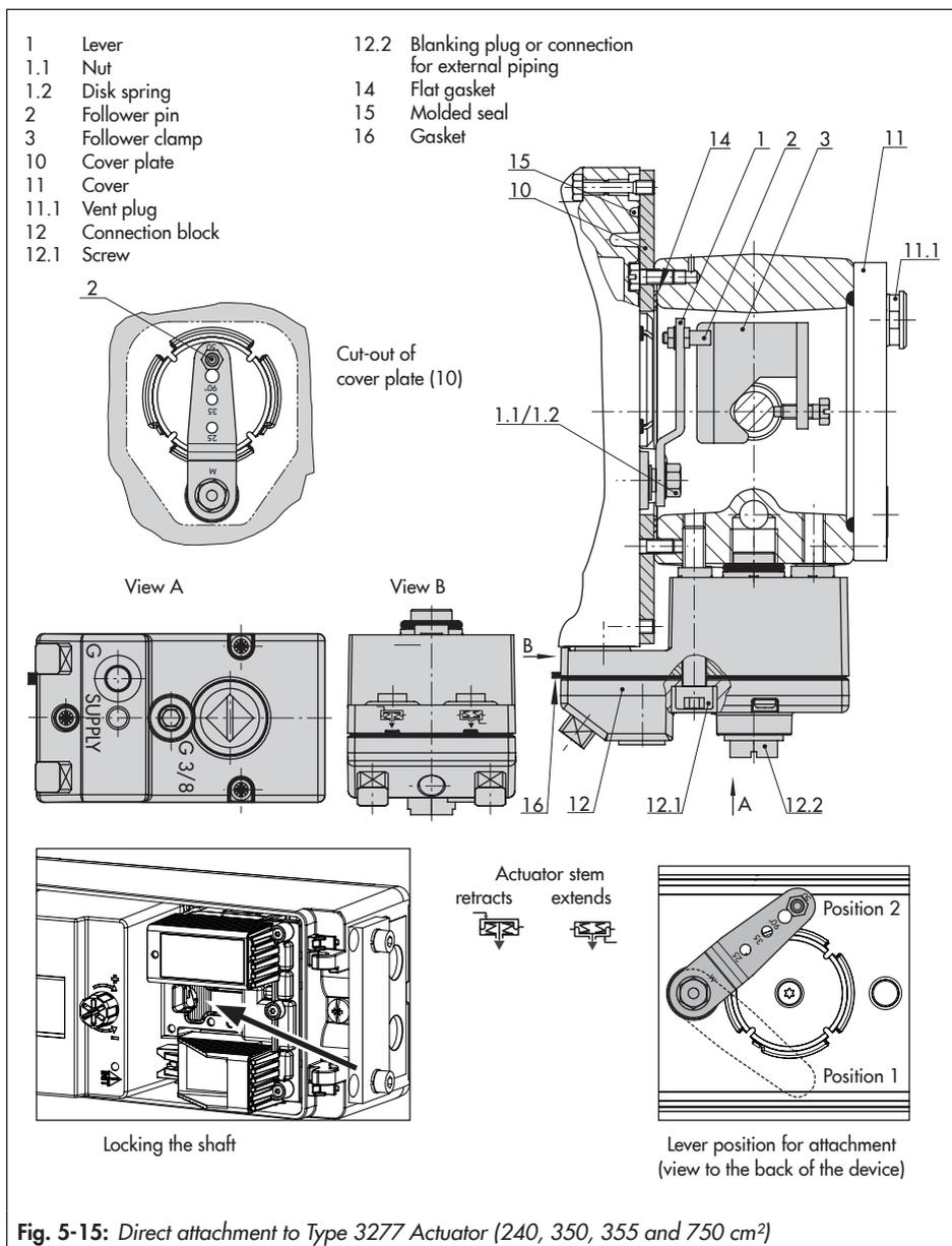
Fig. 5-15: Direct attachment to Type 3277 Actuator (240, 350, 355 and 750 cm<sup>2</sup>)
