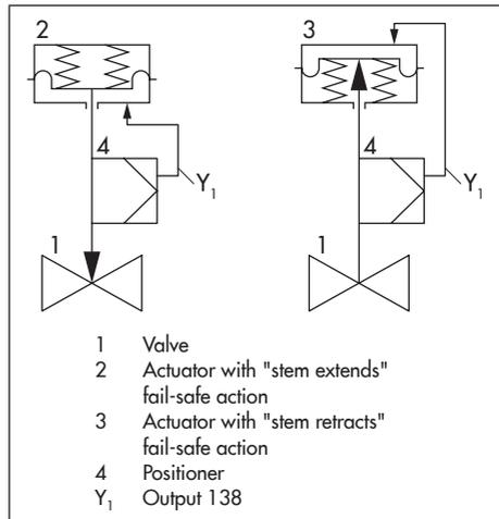
**Typical application with double-acting actuator**
