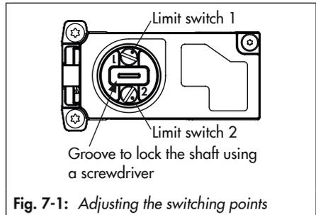
Fig. 7-1: Adjusting the switching points
