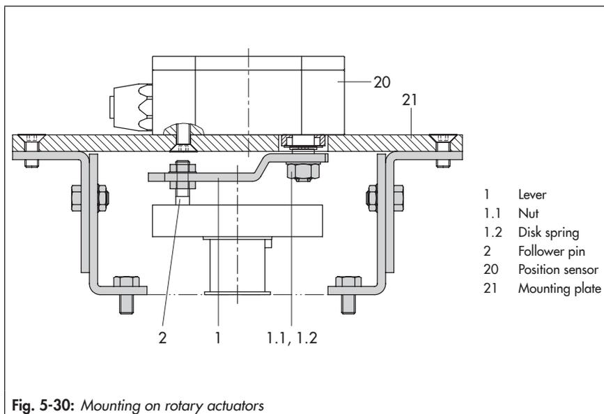
Fig. 5-30: Mounting on rotary actuators
