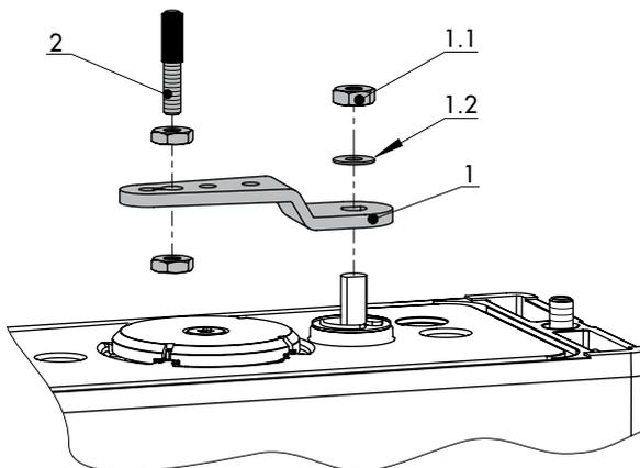
Fig. 5-4: Mounting the lever and follower pin
