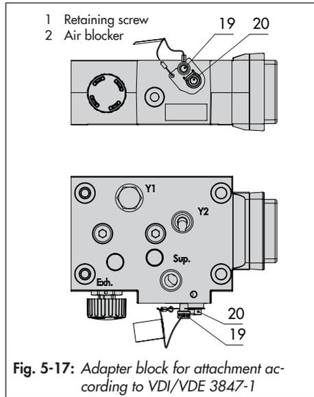
Fig. 5-17: Adapter block for attachment according to VDI/VDE 3847-1
