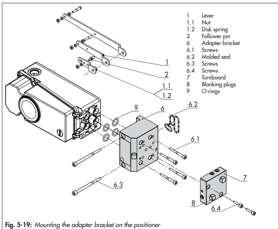
Fig. 5-19: Mounting the adapter bracket on the positioner
