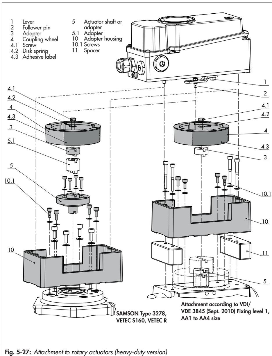
Fig. 5-27: Attachment to rotary actuators (heavy-duty version)
