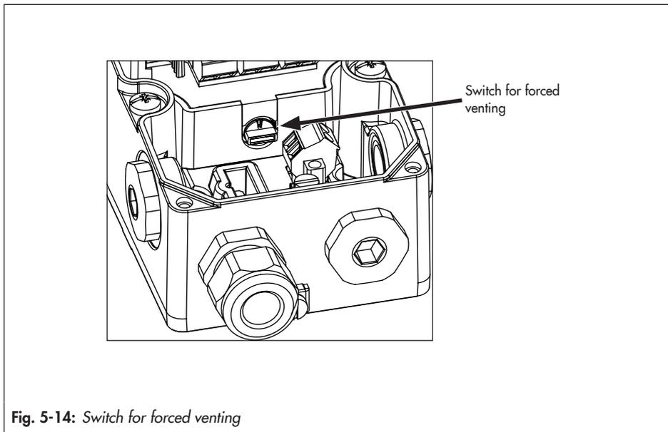
Fig. 5-14: Switch for forced venting
