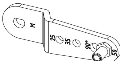
Fig. 5-3: M lever with pin position 50
