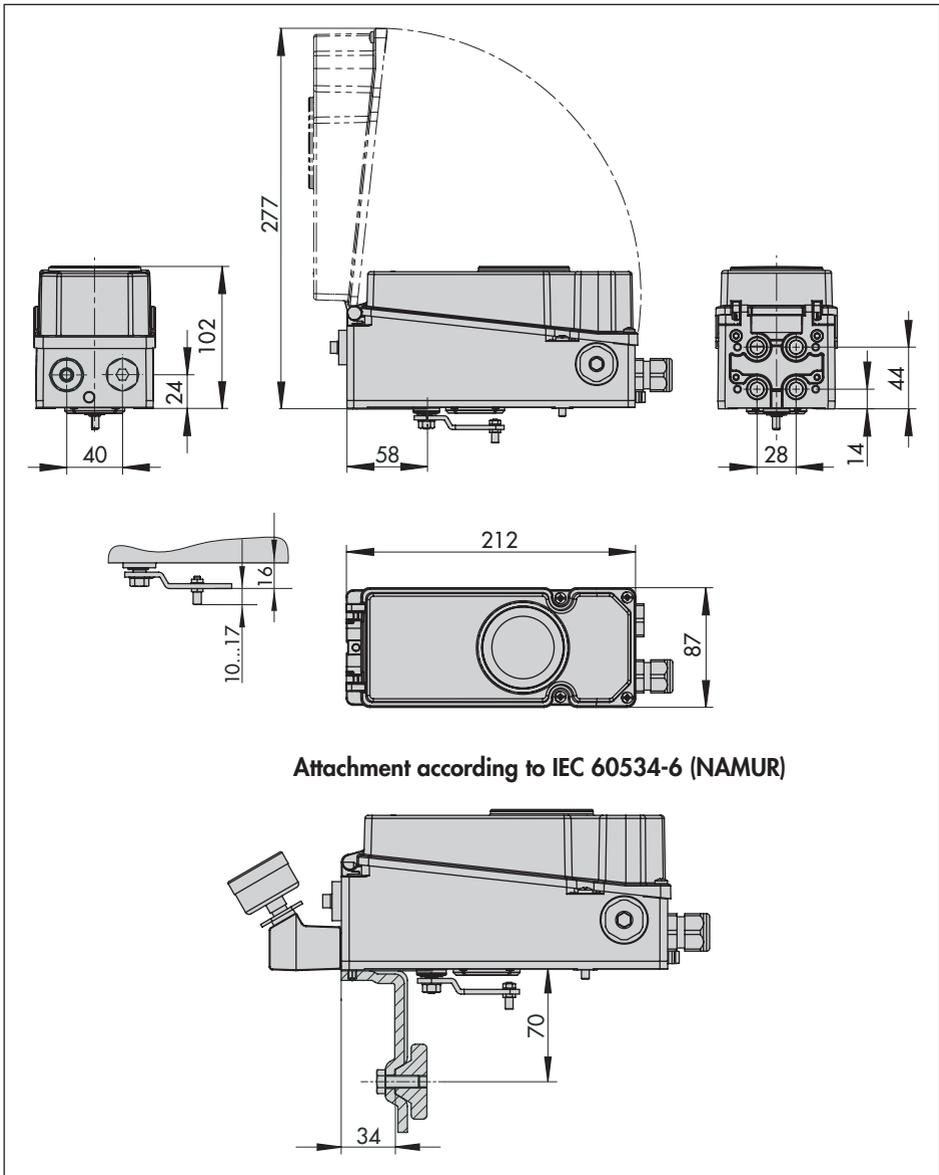
Pressure gauge bracket, two pressure gauges
