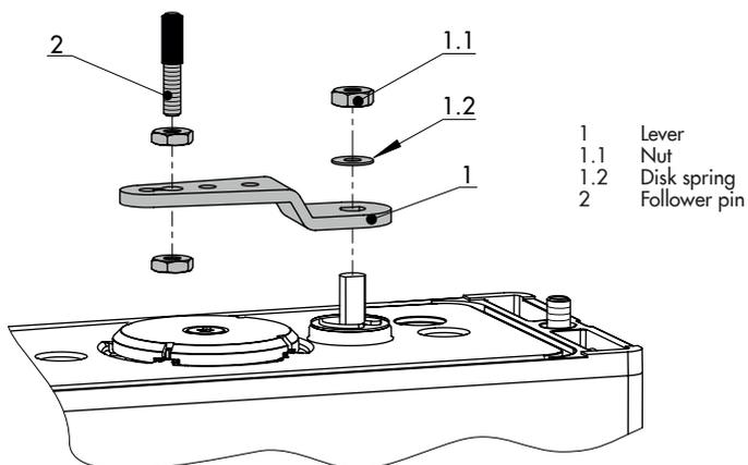
Fig. 5-4: Mounting the lever and follower pin
