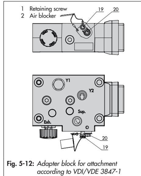
Fig. 5-12: Adapter block for attachment according to VDI/VDE 3847-1
