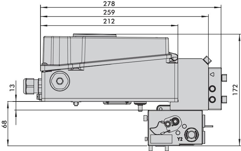
**Attachment to rotary actuators according to VDI/VDE 3845**
