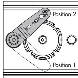
Lever position for attachment (view to the back of the device)
