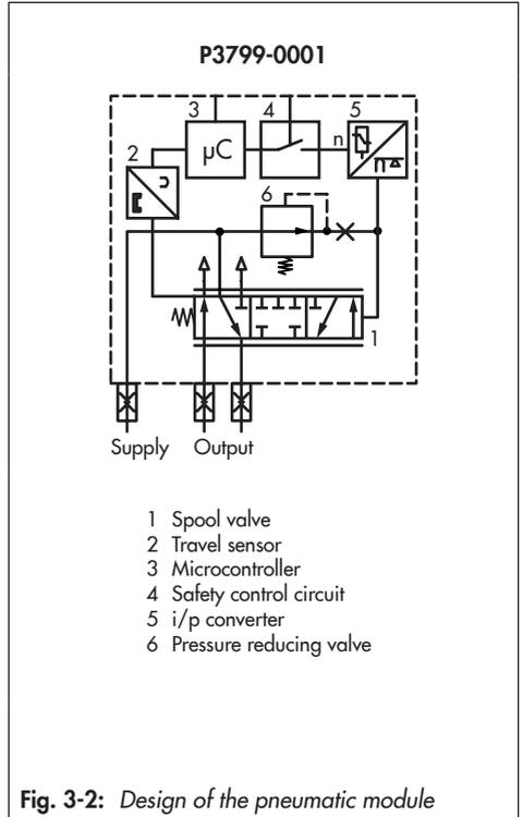
**Fig. 3-2:** Design of the pneumatic module
