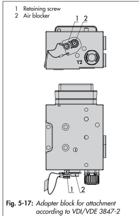
Fig. 5-17: Adapter block for attachment according to VDI/VDE 3847-2
