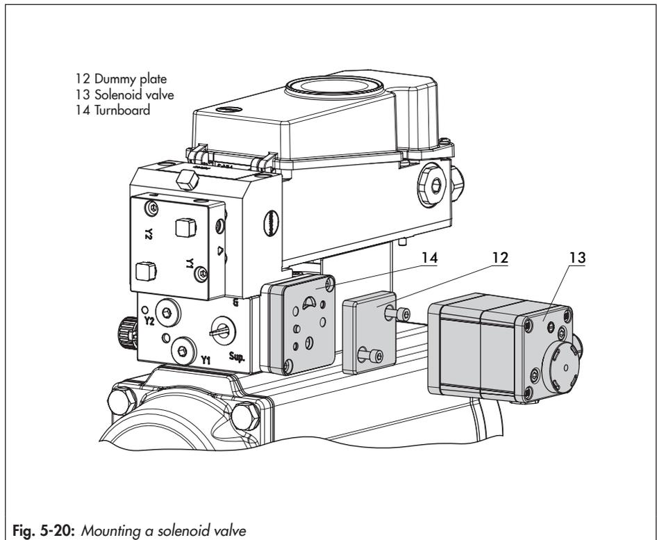
Fig. 5-20: Mounting a solenoid valve
