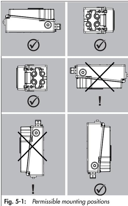
Fig. 5-1: Permissible mounting positions
