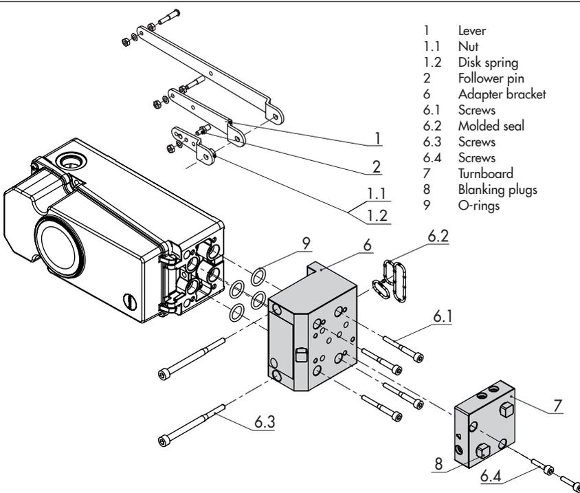
Fig. 5-14: Mounting the adapter bracket on the positioner
