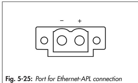
**Fig. 5-25:** Port for Ethernet-APL connection
