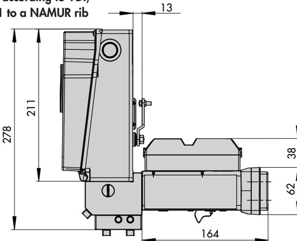
**Attachment to rotary actuators according to VDI/VDE 3847-2**
