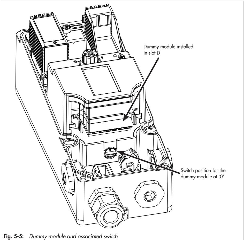
Fig. 5-5: Dummy module and associated switch
