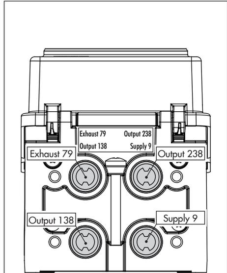
Fig. 5-23: Pneumatic outputs
