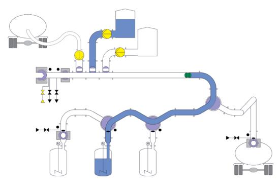
pigs and they are moved through the pipeline as a pair. This can reduce medium residues to the p.p.m. range.
