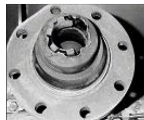
Fig. 21: Damage due to a rotary plug body due to cavitation v_2 \gg 5 m/s.
