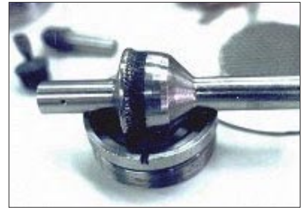
Fig. 19: Typical damage due to cavitation if pressure differential > 20 bar. Feedwater control valve mismatched for start-up 70 to 1 bar.
